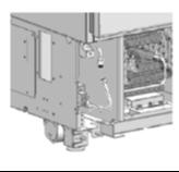
If the appliance(s) is not connected through the side profile trims to secured cabinetry, anti-tip brackets must be installed. The max weight for the cabinet panel is 35 lbs (16kg) for the refrigerator door and 20 lbs (9kg) for the freezer door. For a flush installation, cabinet panels should not be thicker than 15/16".
